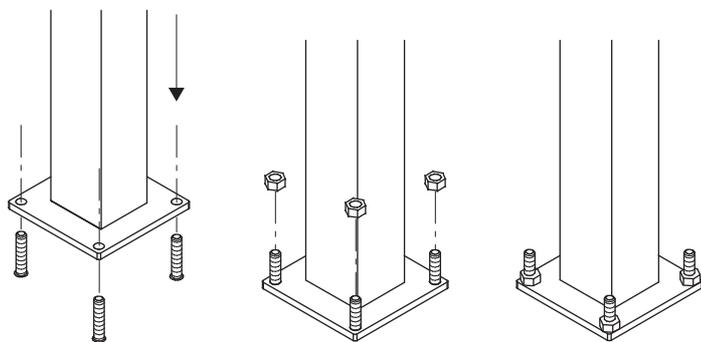
Mount the stainless steel square section post on to the fixing block by means of the useful handling ring fitted to it; eventually tighten the four stainless steel M16 blind nuts.
