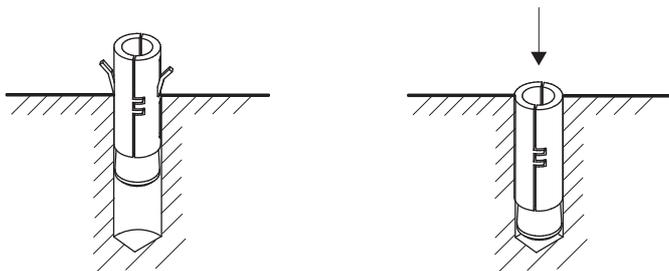
Fit the four M16 stainless steel threaded bolts to the four fixing steel inserts and screw them to jut out 35 to 40 mm; tighten the M16 stainless steel nut so that the bolt can fit the insert very firmly jutting out approx. 45 mm max. from pavement level.
