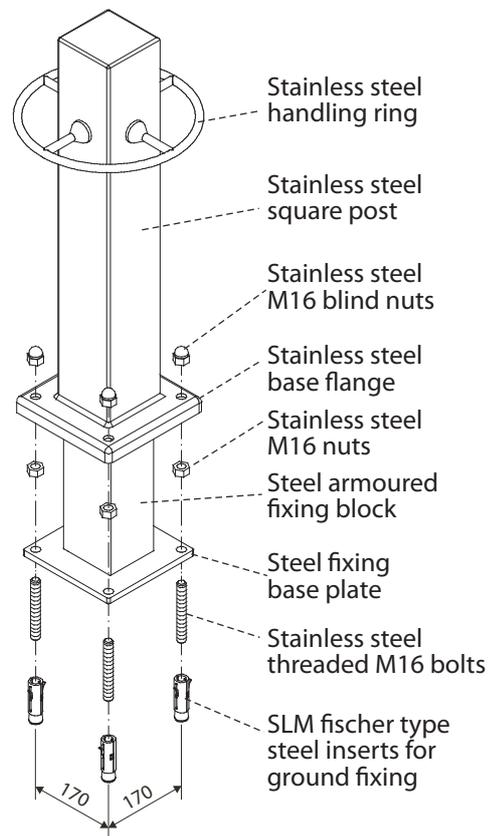
Position the fixing block, armoured core with base plate, on to the four stainless steel bolts; fasten it by tightening the four M16 stainless steel nuts very hard.
